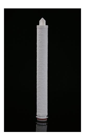
Graded density, high porosity, SPUNFLOW QN filter elements are manufactured from thermally bonded Polypropylene microfibers. Offering high throughputs, low pressure loss, high dirt capacity and long onstream life, the bonded fibre construction minimizes any possibility of fibre migration and is rugged enough to resist particle shedding, even under pulse conditions.
