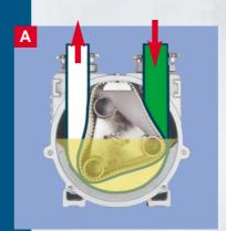
The rotor turns inside the tightly fixed separator. Which is held in the pump housing filled with lubricant. The separator divides the housing into two completely enclosed areas. This means during compression of the pumping hose the suction and discharge sides are hermetically separated.
