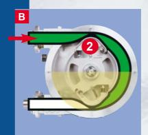
Once the second sliding shoe (2) compresses the hose, a completely enclosed pumping chamber is formed. This volume corresponds exactly to half the pump capacity per rotation. A vacuum is also generated inside the pump housing, supporting the elasticity of the hose allowing restoration to its original full cross-section.
