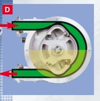
With each rotation the pumping chamber is reformed and the suction capability is renewed.
