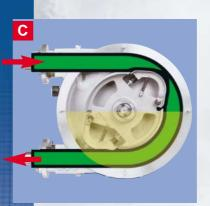
The rotation of the rotor forces the pumped medium inside the hose towards the outlet port on the discharge side. During each opening of the hose a vacuum is created on the suction side ensuring constant suction. It also takes place when the hose is empty giving high suction conditions.
