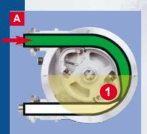
The rotor rotates within the pump housing filled with lubricant and compresses the pumping hose with the sliding shoe (1). This process generates a hermetic separation between suction and discharge side.
