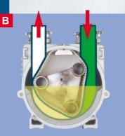
Air from the suction side is pumped over the separator by the turning of the rotor and exhausted outside the pump. This forms a vacuum inside the pump chamber relative to the suction lift, which supports the elasticity of the hose during restoration to its original full cross-section.
