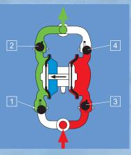
B The control valve switches over the air flow into the left-hand air chamber (blue), the right hand air chamber is exhausted. The suction process (see A) now takes place in the right hand pump chamber. Medium (red) is drawn in. Medium (green) is pressed out of the left-hand pump chamber. Valve ball (1) is pressed down and closes, whereas valve ball (2) opens allowing the medium to flow to the outlet.
