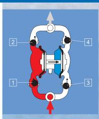
By filling the right hand air chamber with air (blue) the righthand diaphragm is pushed outwards. This pulls the piston rod on the left-hand diaphragm to the initial position. The valve ball (1) is drawn out of its position, the medium (red) flows into the left-hand pump chamber. At the same time valve ball (2) is seated in a closed position by the vacuum. The left-hand pump chamber fills up with medium (red).
