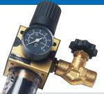
If only poorly treated compressed air is available, DEPA air operated diaphragm pumps should be fitted with an upstream service unit. The special filter in service unit almost completely cleans the compressed air from residues of water and oil droplets. The integrated pressure regulator maintains the working pressure at an almost constant level, independently from pressure fluctuations in the mains air supply.
