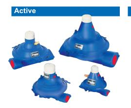
DEPA air operated double diaphragm pumps can be equipped with an active pulsation dampner installed immediately after the pump. This reduces any remaining pulsations to a minimum.
