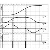
Effect of the feedforward measures using the jerk feedforward as an example without feedforward jerk control with feedforward jerk control
