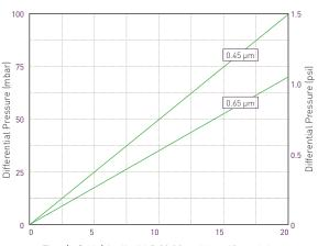
Flow (L / min) for liquid @ 20 °C and 1 cp 10"module Recommended beer flow rate of 1.5-3l/min/10"module
