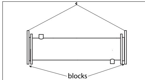
**⚠ Attention once removed the safety plates, keep the aftercooler always horizontal and avoid tilting the aftercooler which will cause the tube bundle or the sealing rings to fall out, with consequent risk to person or property.**
