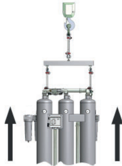
II: Installing by crane
