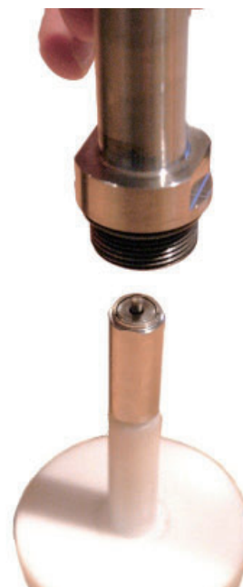
Valve armature gauge
