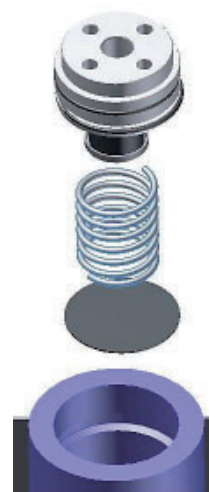
Piston, dust screen, spring and perforated plate
