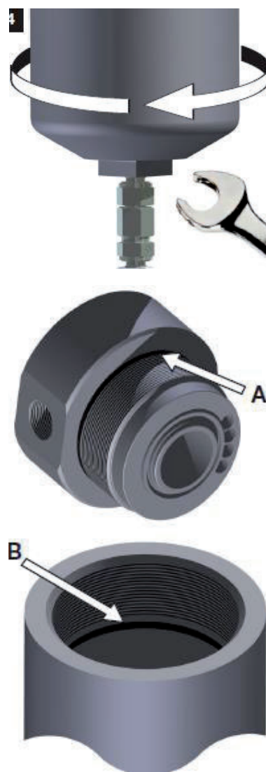
Changing filter elements
