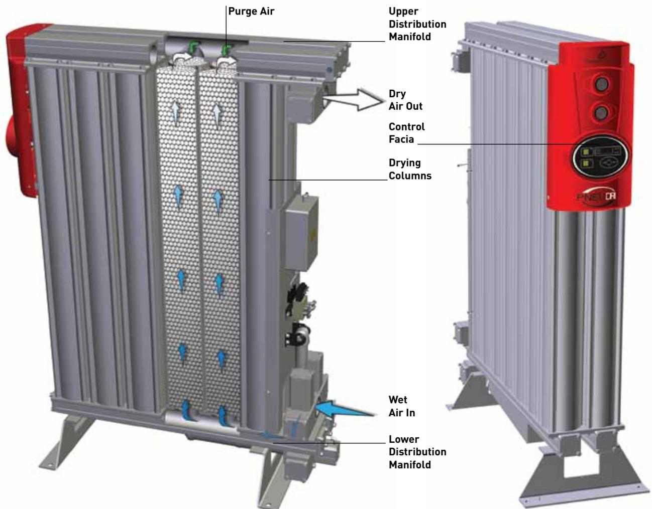
One chamber is operational (drying), while the opposite chamber is regenerating using either the Pressure Swing Adsorption (PSA) (heatless) or Thermal Swing Adsorption (TSA) (heat regenerative) method of drying.
