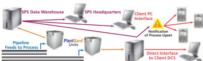
Continuous measurement and surveillance of gas stream cleanliness, data logging, report generation and remote alarm notification via Web, DCS, or mobile telephone – 24/7
