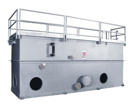
These plates are mounted in modular packs and provided with an adjust device against the vessel which insures that all the flow to be treated goes through the Plates. Optimal working range temperature of Plate Packs MPak® is 4 to 98 °C (40 to 208 °F). Each oil separator of the MAS Series can be equipped with adjustable skimmers to withdraw separated hydrocarbons. Optionally, they can also be provided with a storage chamber to accumulate separated hydrocarbons.
