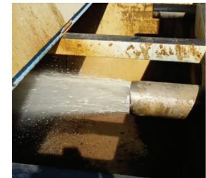
The pictures above show the backflush cleaning process of the BlastPure system. The dirty, contaminated water is literally blasted off the metallic filter cartridges during the cleaning cycle. The water color coming out from the blast goes from dark to clear as the filter cartridges are cleaned and prepared to be put back online.
