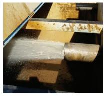
The pictures above show the backflush cleaning process of the BlastPure system. The dirty, contaminated water is literally blasted off the metallic filter cartridges during the cleaning cycle. The water color coming out from the blast goes from dark to clear as the
