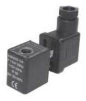
This miniature coil is designed for valves equipped with a miniature tube assembly (2000 series valves). This is an encapsulated assembly comprising a coil, integral magnetic iron path and snap-on plug connection. The synthetic material encapsulation provides an effective compact housing, offering full protection against dust, oil, water, etc. Ease of mounting in confined space - offers shock and corrosion protection - simplifies conversion of existing equipment to other requirements, etc.
