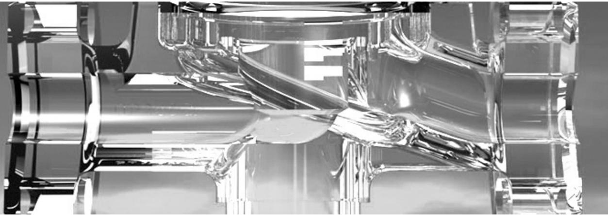
Force pilot operated valves operate from 0 bar and can be installed where directly acting valves are used. However, beyond the range of the latter, they are supplied with smaller solenoids for higher pressures and larger nominal sizes. The actuator of a force pilot operated valve opens a pilot orifice and then lifts the sealing element from its seat directly or supported by the delta p of the operating pressure.
