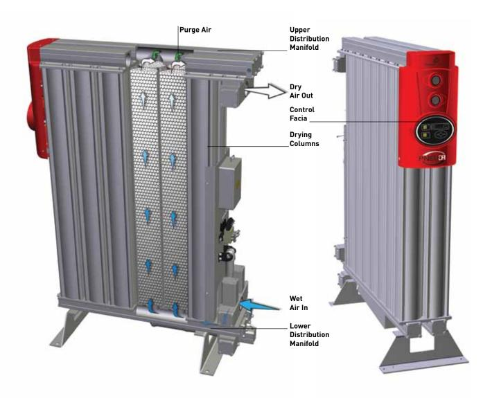
One chamber is operational (drying), while the opposite chamber is regenerating using either the Pressure Swing Adsorption (PSA) (heatless) or Thermal Swing Adsorption (TSA) (heat regenerative) method of drying.
