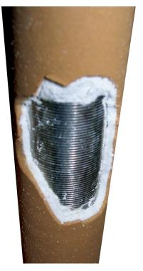
A sample of the uniformly floated individual layers of kieselguhr on the candle.
